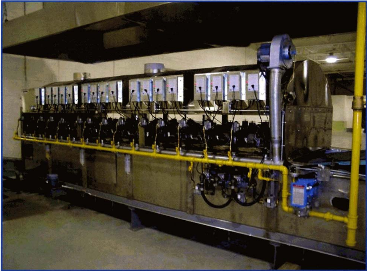
Burner Buddy® Flame Safety and Ignition Systems on a Bakery Oven Application
