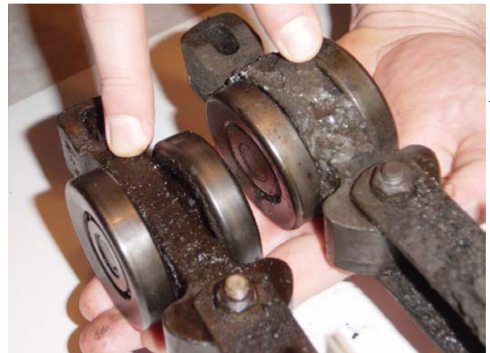
After Cleaning (Left) & Before Cleaning (Right)
